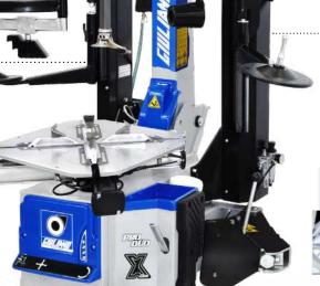
Equipped with Help and Press Arm powerful pneumatic helper systems, to enhance tyre changer's performance and provide a valuable support in mounting/demounting most difficult tyre applications in the market, such as Run Flat, UHP and low profiled tyres.
